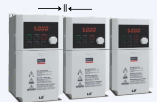
Side-by-side installation (2mm between drives)
